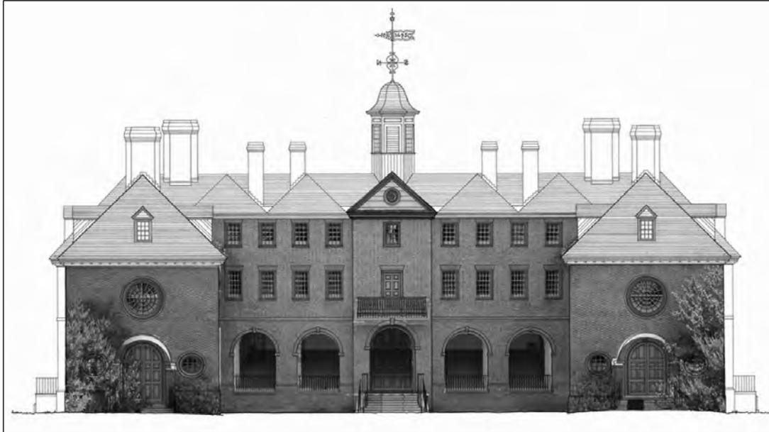
The images on this page illustrate the process of creating hybrid drawings, a blend of measured drawings and high-resolution photographs taken from multiple points of view. Shown are five survey photos and a HABS drawing of the Sir Christopher Wren Building on the campus of the College of William & Mary in Williamsburg, Virginia. Frazier Associates of Staunton, Virginia, rectified and scaled these photographs for integration with the measured drawing to create the hybrid elevation drawing shown.
