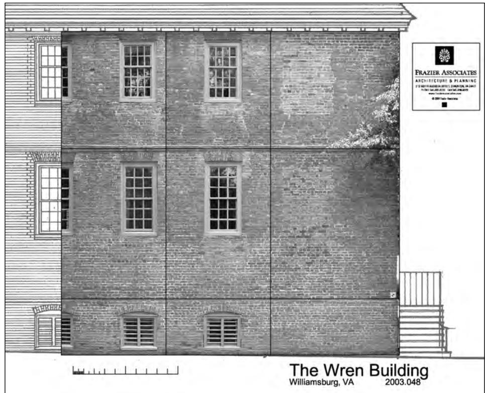
This portion of another hybrid elevation drawing of the Sir Christopher Wren Building illustrates how a measured drawing can be combined with survey photographs to add a record of material condition data to the dimensional data recorded in the drawing.
