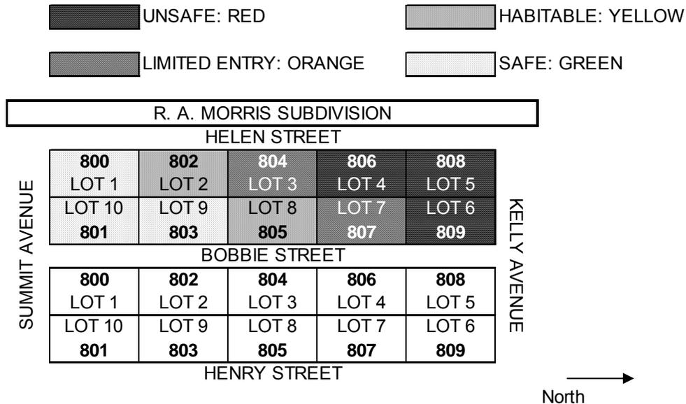
The example given is the inspection made after a tornado struck Block One of the R.A. Morris Subdivision. If North is to the right of the subdivision, we can trace the path of the tornado and the damages it caused. In this case, the tornado was moving from the Southwest to the Northeast.
