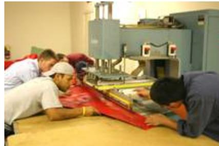
*UTSA students "welding" fabric panels using Chism Company's Radio Frequency Welder.*
