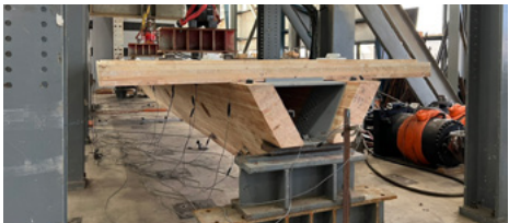
V-cassette testing at Oregon State University
