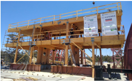
Above: Two story initial full scale test in 2017 Left: Ten story final test in 2024
