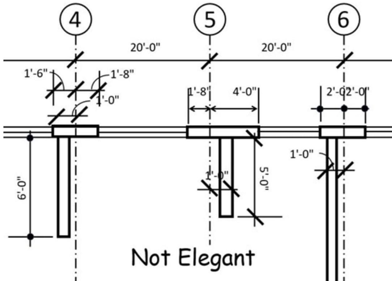
Even a plan that follows all the above tips can still look ugly and messy. Thus, the final step in creating well-dimensioned plans is organizing the dimension strings so they elegantly provide information without cluttering the drawing. Provide all the necessary dimensions in the fewest possible number of strings, and avoid scattering the strings randomly throughout the plan. Make the plan drawing look good as well as be informative.
