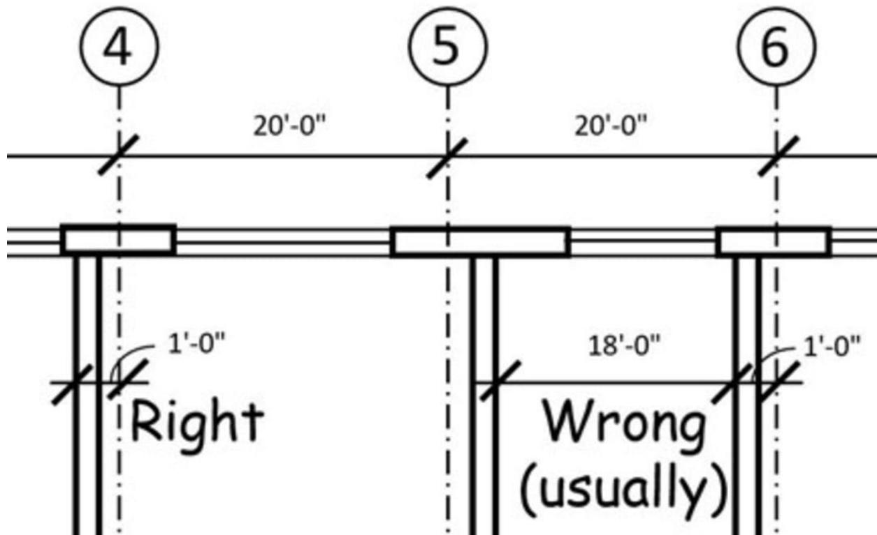
Don't dimension the clear widths of rooms unless they're important. In most cases they aren't, so just locate one face of each partition to its nearest column line.
