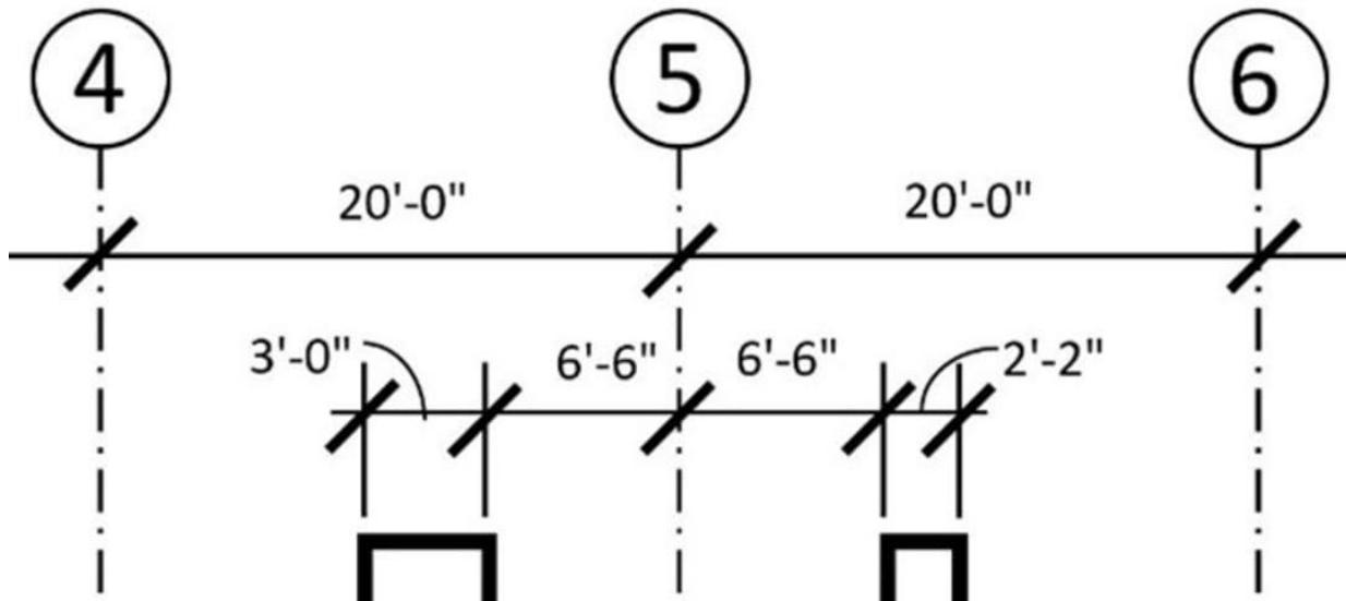
Column center lines are the starting points for all strings of dimensions.<sup>2</sup> You should be able to trace every dimension to its closest column line. (For renovation or tenant improvement projects where column lines don't exist or can't be precisely located, use fixed elements, such as faces of existing walls, as the starting points for dimensions.)
