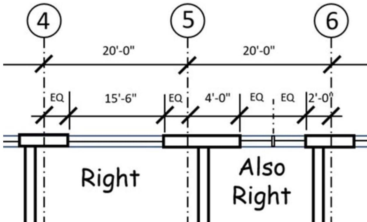
Some dimension strings might be called **semi-closed** (or, for optimists, semi-open). This occurs when two or more dimensions within the string say “Equal” instead of a “X-X”.<sup>4</sup> Use “Equal” when you want two or more dimensions to be the same, but the precise dimension doesn’t matter. Remember that “Equal/Equal” works only if every other dimension within a known length is identified.
