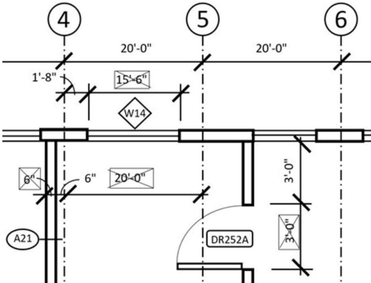
The purpose of dimensioning, like every other aspect of the construction drawings, is to give the contractor just enough information to build the project, and—ideally—not a bit more than that. In the case of dimensions, every element of a floor plan should be locatable through just two strings of dimensions (one for each direction). When dimensioning, think minimalist. Every dimension should serve a purpose, and no other dimension should be serving the same purpose.
