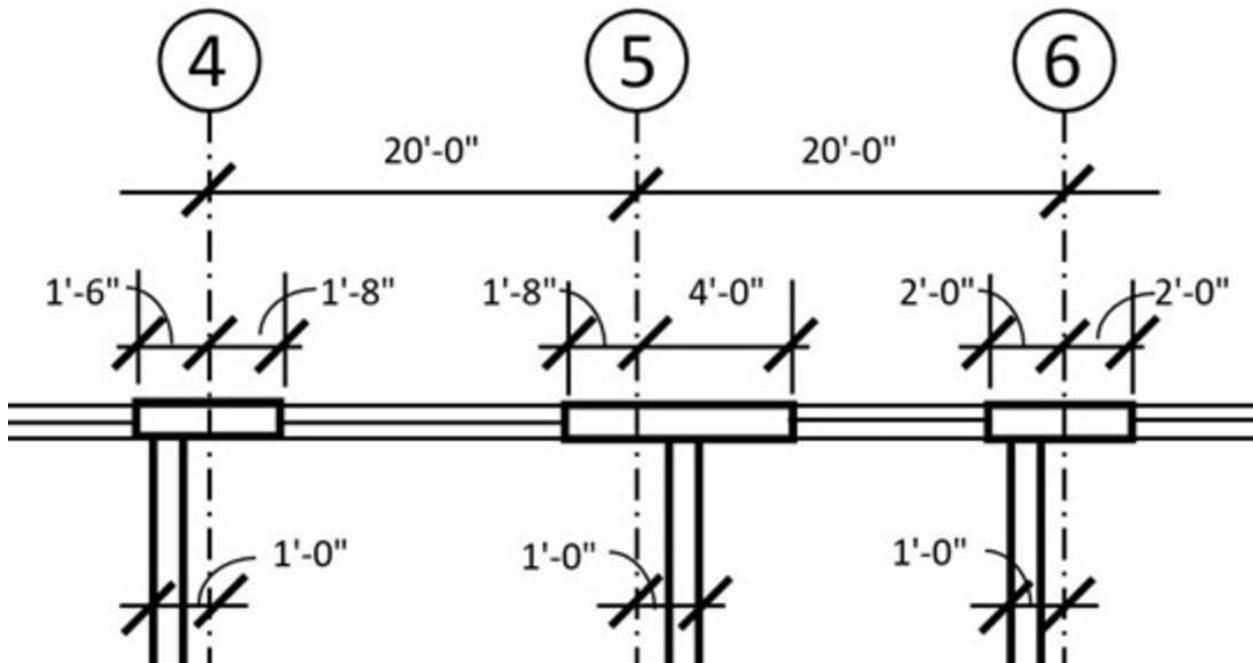
Keep dimensions of column lines and exterior building elements, such as piers and window openings, outside the floor plan, while interior dimensions should be located inside the floor plan. This prevents clutter and confusion. Place the column line dimension strings along the top and the right-hand sides of the sheet, where they can be most easily found and read.
