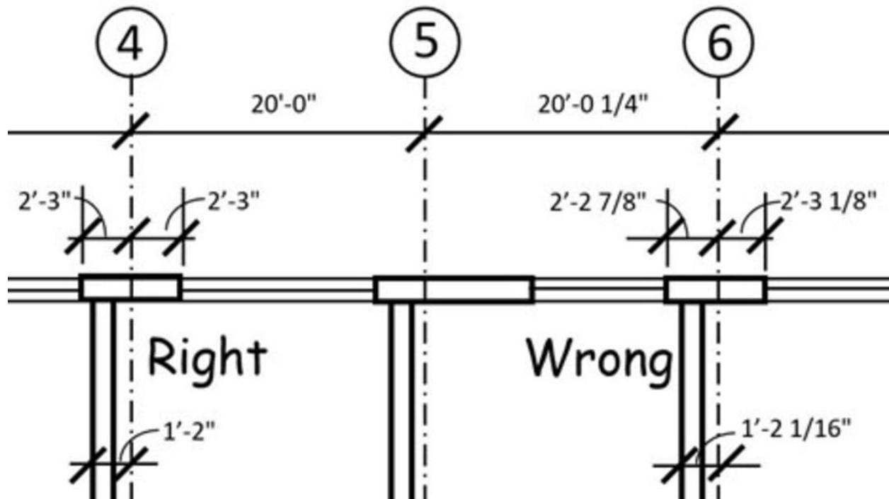
Every aspect of construction is governed by tolerances and degrees of precision. Work built in a shop under controlled conditions, such as millwork, can be built with considerable precision, while work built on site under whatever conditions are prevailing at the time of construction can be built much less precisely. When we dimension, we have to allow for these construction tolerances or our drawings won't be buildable.
