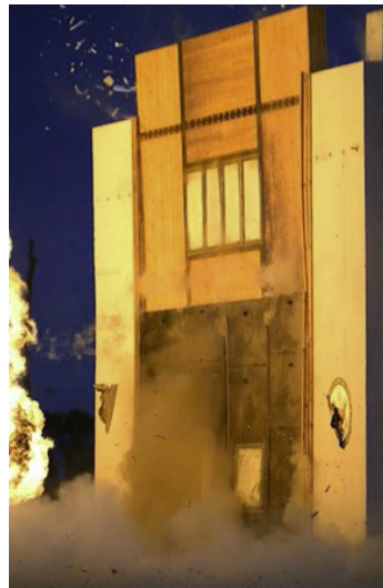
Blast testing mass timber mock-up with digital assessment of impacts
