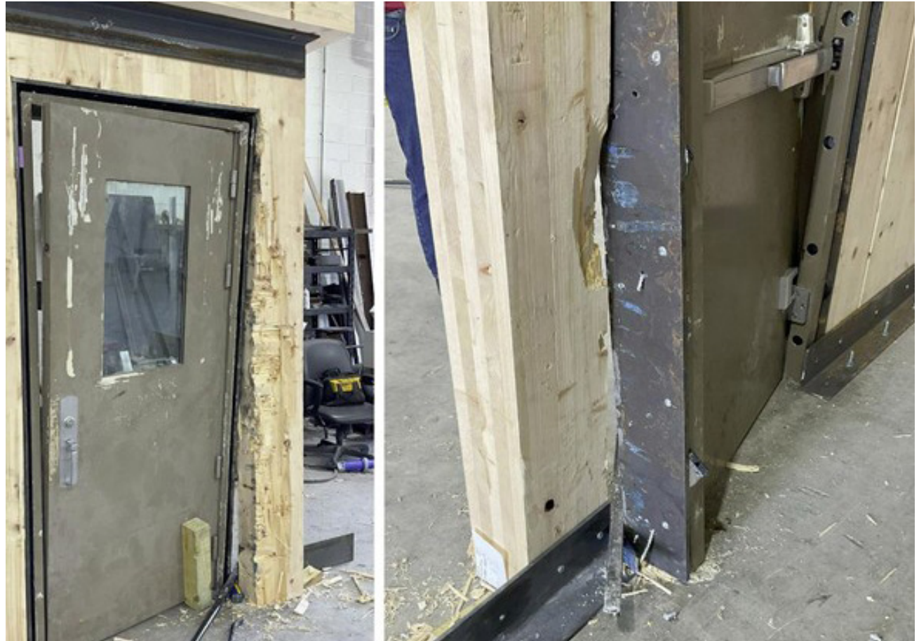
Forced entry testing of mass timber assembly
