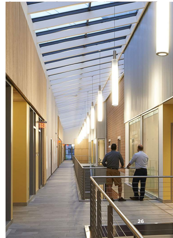
Daylighting analysis of the atrium meets IES targets (50 lux – circulation, 300 lux – work areas), with adopted recommendations including transom windows to improve daylighting in work areas and solar reflectors on existing walls to enhance sunlight penetration.
