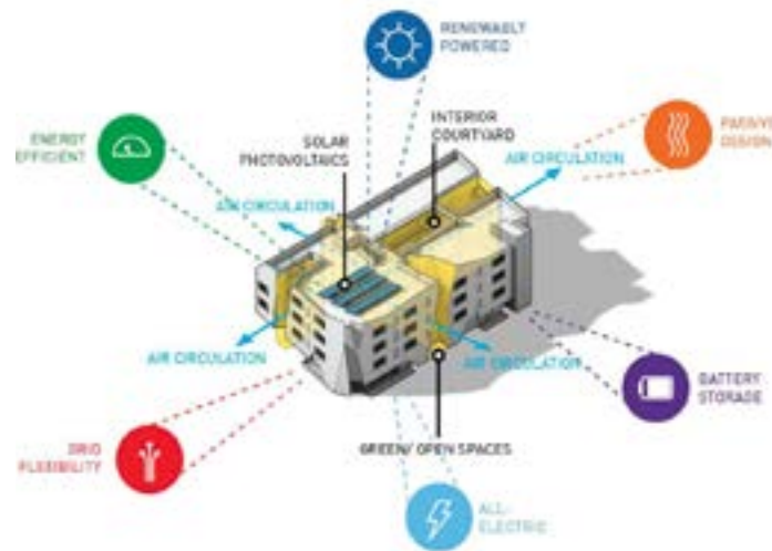
Pacific Landing has a measured Energy Use Intensity (EUI) of 7.1 kBtu/sf/yr, an incredible 46% reduction in energy, not including the on site rooftop solar which generates 37% of the buildings electricity. Diagram Credit: Patrick TIGHE Architecture; Copyright: Patrick TIGHE Architecture
